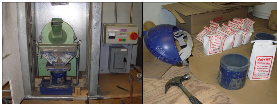
FIGURE 12. SOIL GRINDER AND SAMPLES AT THE UNIVERSITY OF MANITOBA, DEPARTMENT OF SOIL SCIENCE. SOIL SAMPLES WERE PULVERIZED, PACKED, AND SHIPPED TO AGVISE LABORATORIES FOR ANALYSIS.
