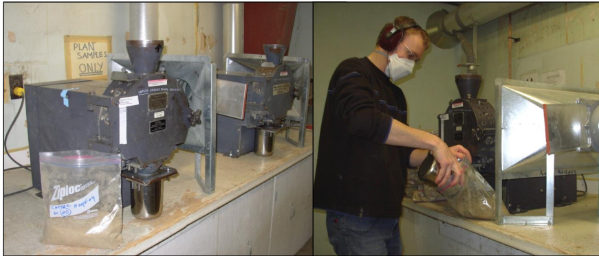
FIGURE 10. PLANT SAMPLE PROCESSING. WILEY MILLS GRINDERS GROUND PLANT MATERIAL TO DUST. SAMPLES WERE TRANSFERRED TO SAMPLE BOTTLES AND SENT TO AGVISE LABORATORIES FOR COMPLETE NUTRIENT ANALYSIS.
