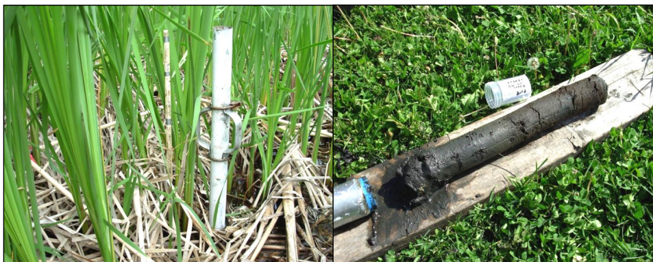
FIGURE 9. SEDIMENT CORER SHOWN INSIDE A 1M X 1M QUADRAT (LEFT); A SUCCESSFUL 5-CM DIAMETER SEDIMENT CORE REMOVED FROM SEDIMENT CORER (RIGHT).
