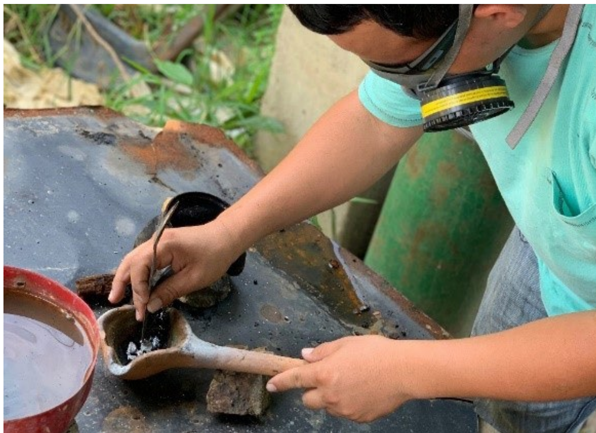
FIGURE 6. Mercury vaporizing conducted by an ASGM operator in La Mina, Honduras
