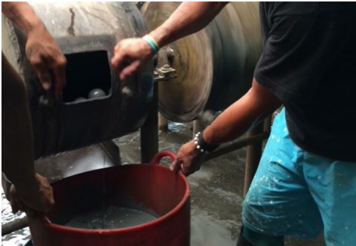
FIGURE 5. Amalgamation barrel in Colombia
