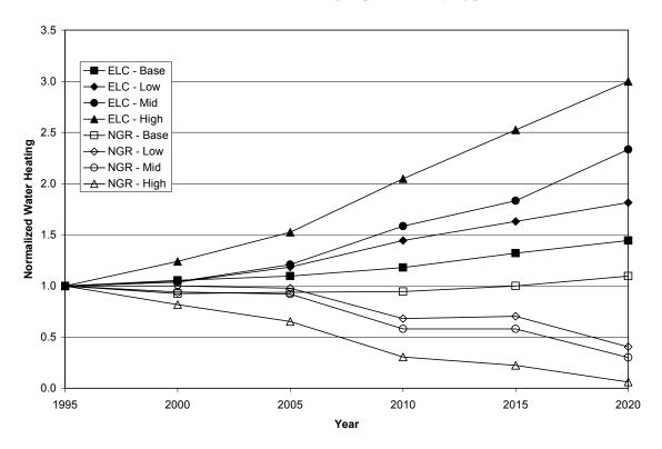
Figure 8: Normalized Water Heating Consumption: Electricity and Natural Gas
