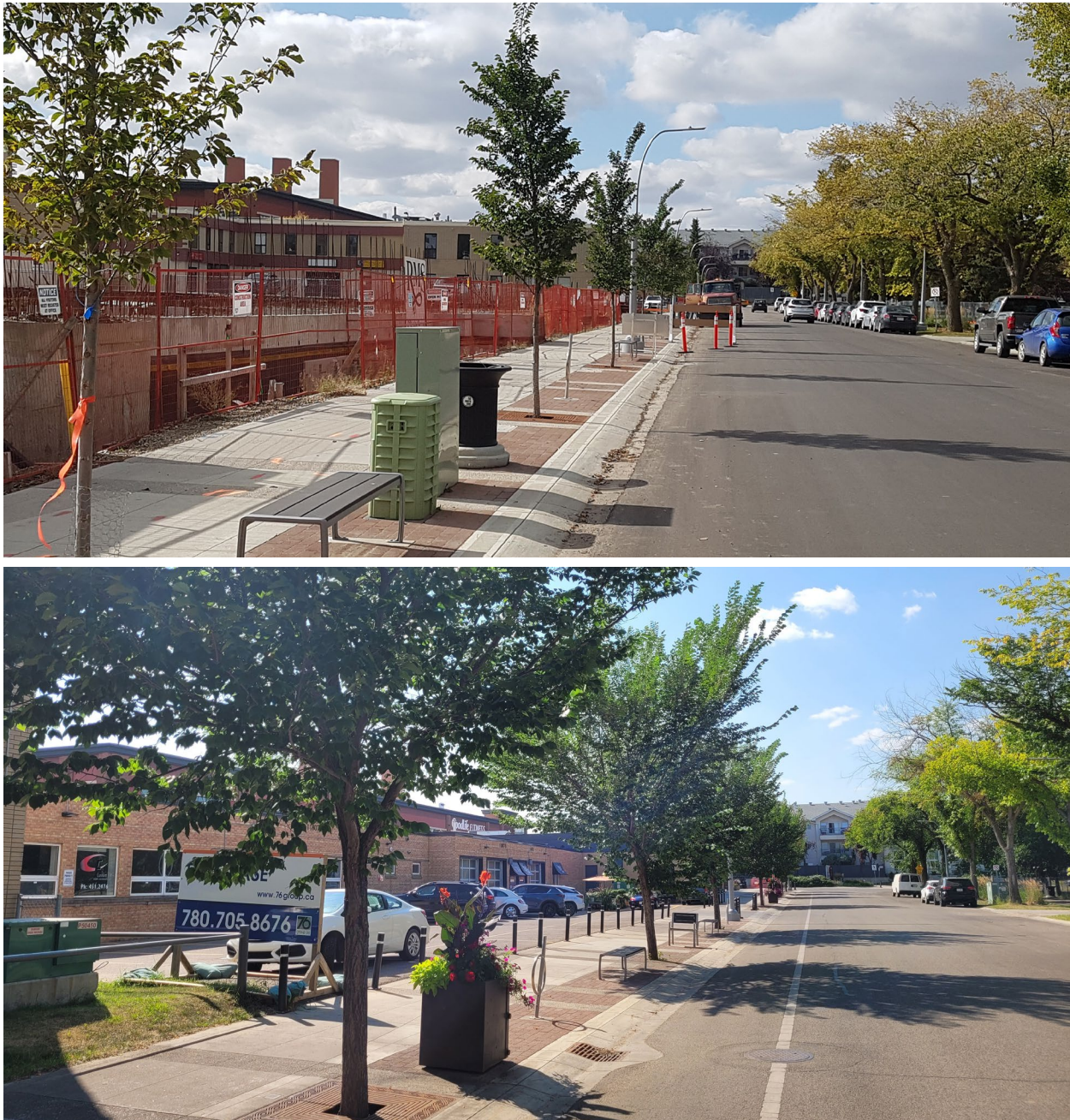
Figure 13. 105th Avenue in the Unity Square area, Edmonton, Alberta, elm trees planted in soil cells (2017) show continuing rapid growth after 5 years (2022)
