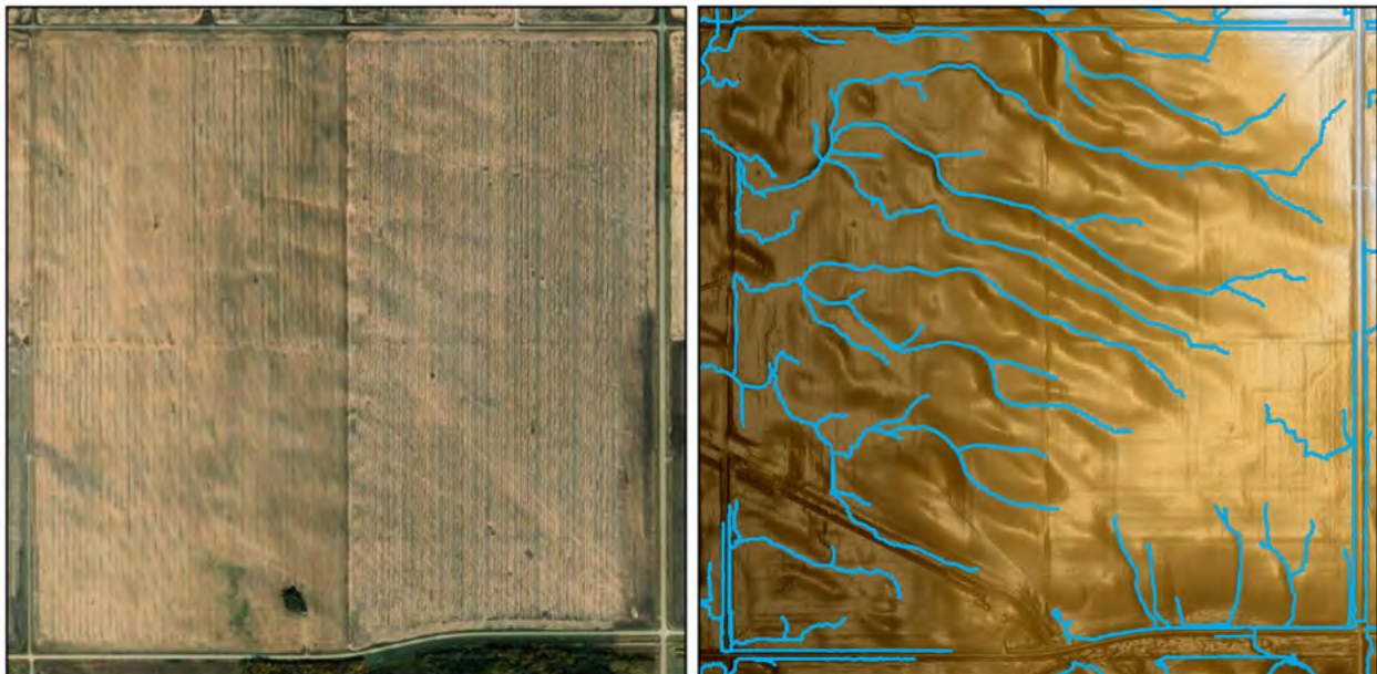
Figure 2. Field-scale flow accumulation analysis using a LiDAR-based DEM (elevation drops primarily from right to left)
