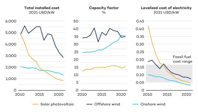
**Figure 4.8** Global weighted average total installed cost, capacity factor, and LCOE of newly commissioned utility-scale solar PV, onshore and offshore wind, 2010–2021
