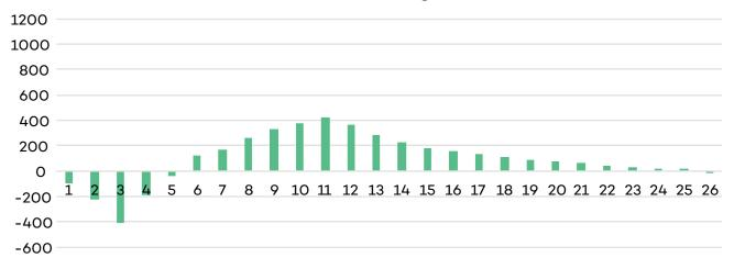
Figure 2. Undiscounted and discounted cash flow of the same hypothetical oil and gas project over its lifecycle (five years for project development, 20 years of production and one year for decommissioning)
